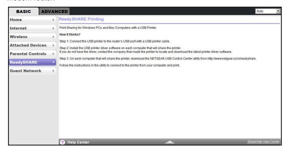
The USB Control Center utility allows you to control a shared USB device such as a printer from your computer that is connected to the USB port on your router.
